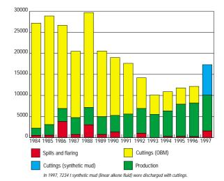
Figure 4.11 Contributions from the different sources of oil input (tonnes) to the North Sea from offshore installations.
