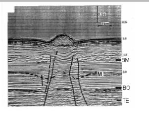
Seismic profile of carbonate mounds and sub-surface fault traces (from Hovland *et al.,* 1994).
