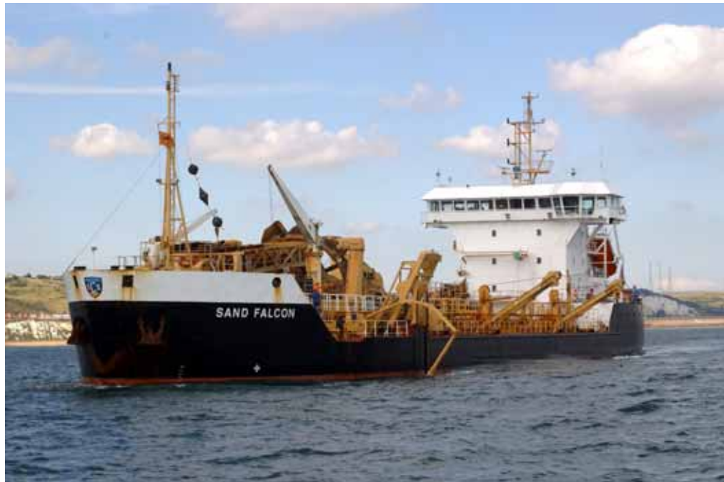
Figure 2.6.1. A typical construction-aggregate trailer suction hopper dredger, the MV “Sand Falcon”. The vessel has a cargo capacity of 5000 m 3 and has both screening towers and a bucket wheel self-discharge system.
