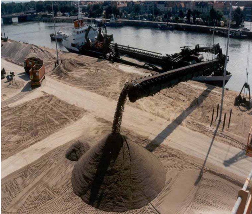
Figure 2.6.2. A typical construction-aggregate trailer suction hopper dredger, the MV "Orisant", discharging at the quay in the harbour of Bruges, Belgium.
