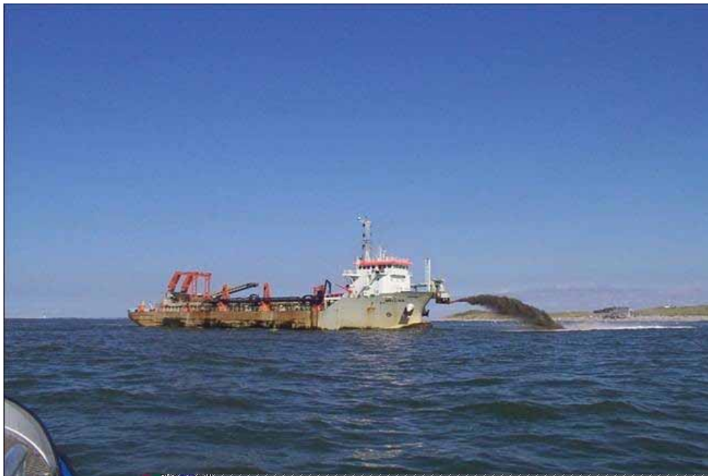
Figure 2.6.3. A typical construction-aggregate trailer suction hopper dredger, the MV "Mellina", supplying sand for beach nourishment at the coast of Ameland, the Netherlands.
