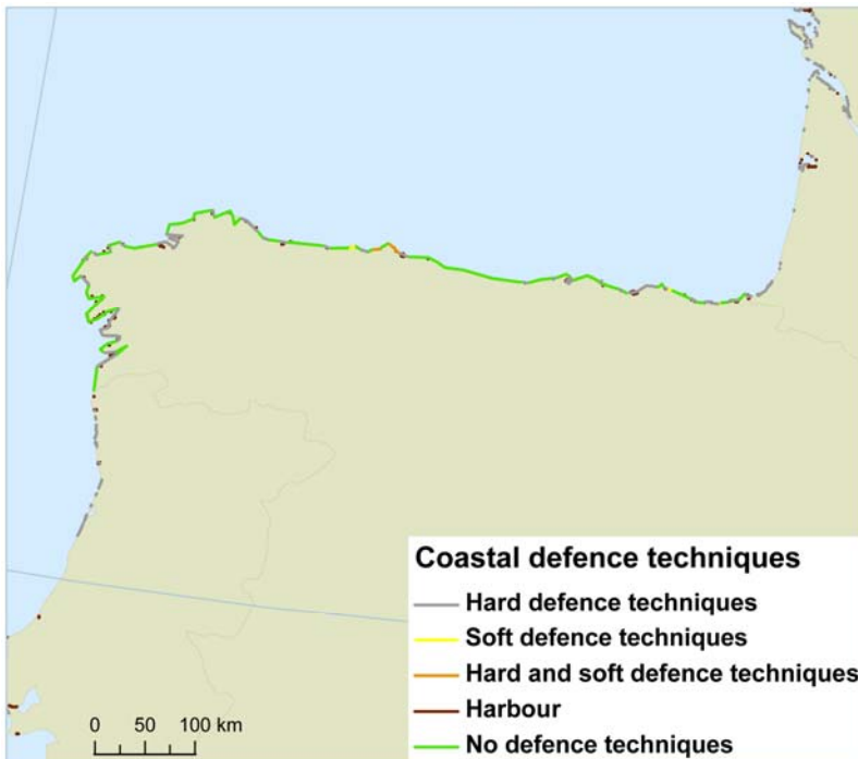
Figure 4: Coastal defence techniques applied in the North of Spain
