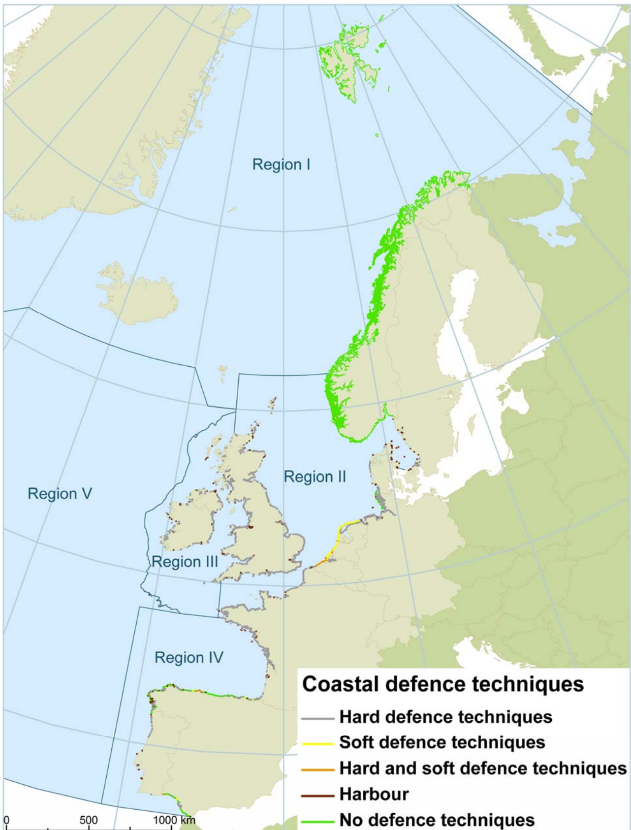
Figure 1: Coastal defence techniques used along the coastline of the OSPAR Maritime Area.
