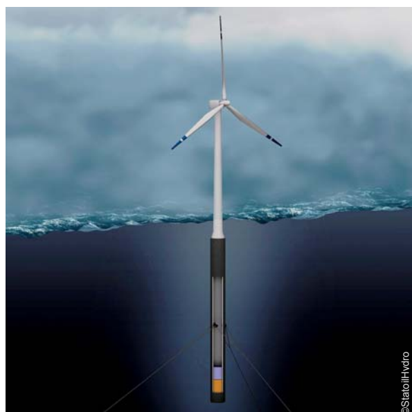
Figure 3.1 Technologies for floating wind turbines are expected to enable wind power generation far offshore at sites with greater water depths. At a test site off Karmøy (southwest Norway) a 2.3 MW wind turbine is attached to the top of a floating concrete buoy construction, which is moored to the seabed, using three anchor points, a system also applied in the offshore oil and gas industry.
